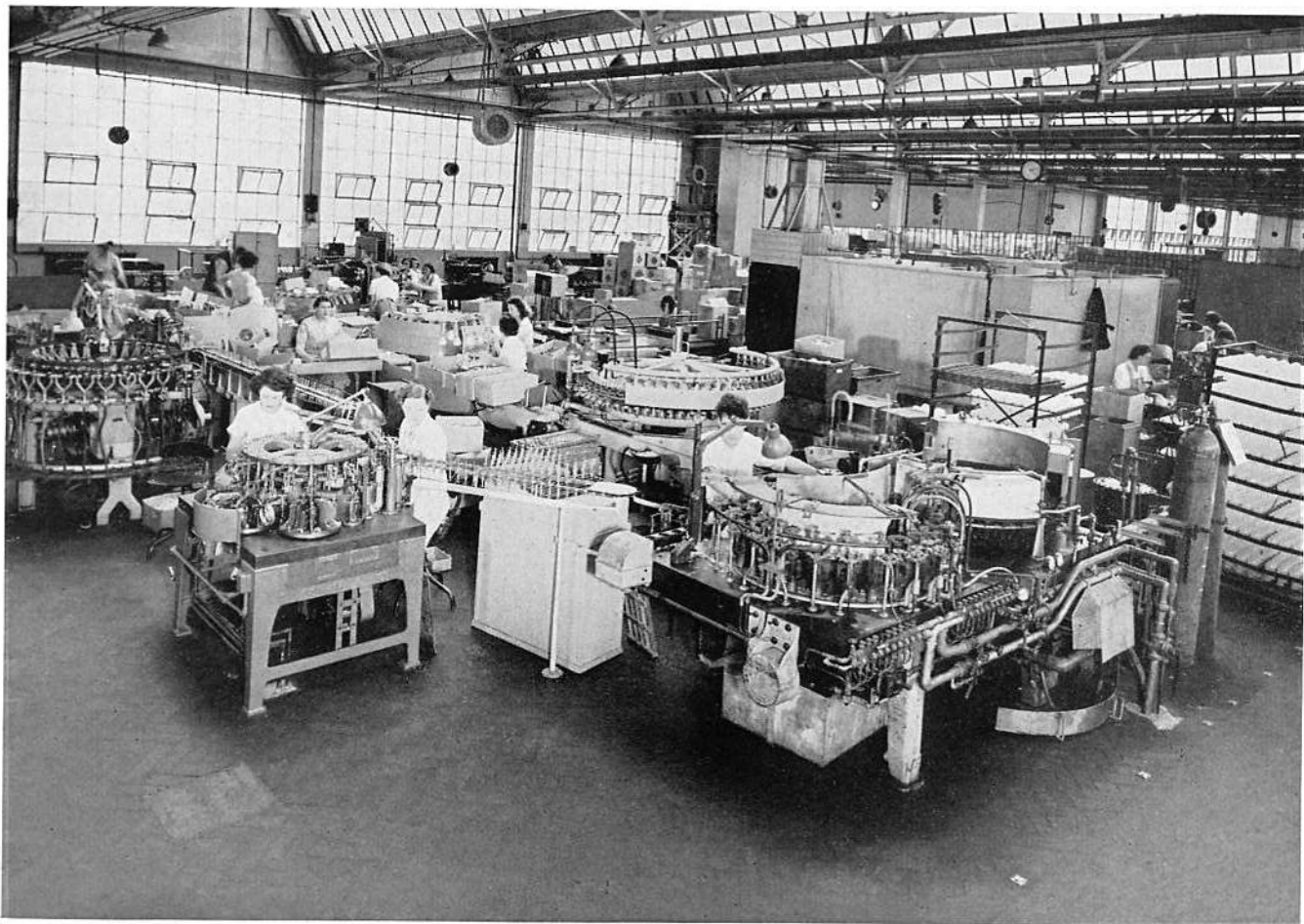
Components are assembled on the machine on the left, and pass to the support and filament-mounting machine (left foreground). After lamps have been exhausted and filled with gas (right foreground) they are capped on the finishing machine (right centre), inspected and packed.
