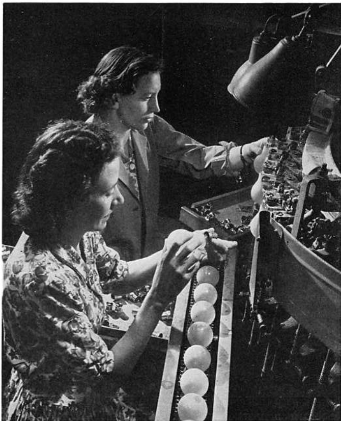
Metal caps are secured to the glass bulb by a special cement, the 'curing' cycle of which is controlled to ensure a bond which resists rigorous climatic conditions.
